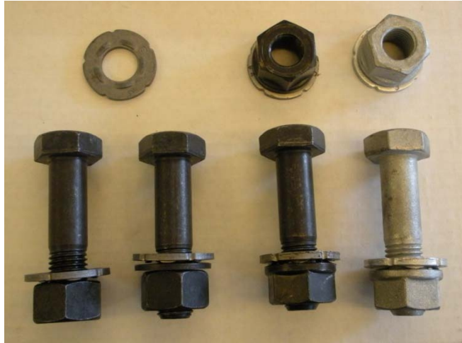
Figure 2. Test configurations from left to right; DTI without washer, DTI with washer, plain TurnAnut DTI, galvanized TurnAnut DTI.
