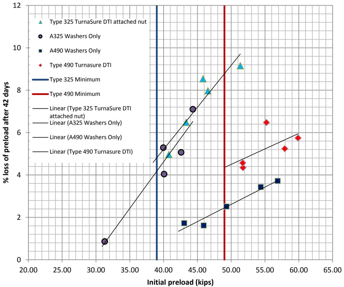
Figure 5. Percent loss of bolt tension relative to initial tension at 42 days.
