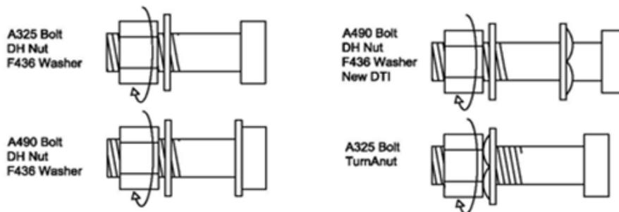
Figure 1. Bolt assembly configurations used in the test procedure.
